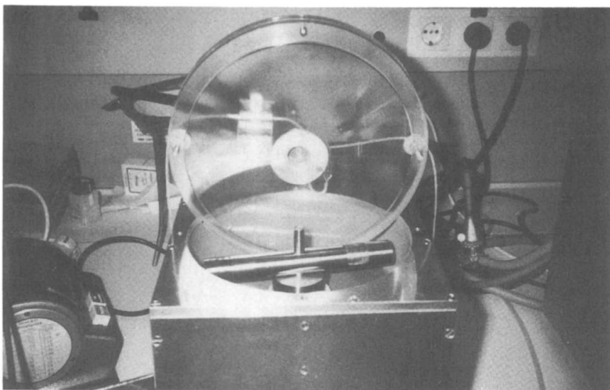
Figure 2: Photographs of the new elutriator ready for operation (upper panel) or partially disassembled (lower panel) showing the steel-tube rotor. (Adapted from ref. 11).
